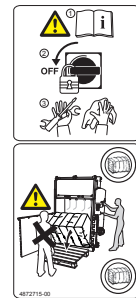
The main power switch must be turned off to « 0 » and secured with a padlock before service or cleaning.
