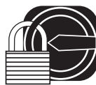
The main power switch must be turned off to « 0 » and secured with a padlock.
