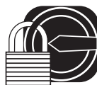
The main power switch must be turned off to « 0 » and secured with a padlock.
