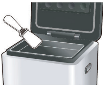
Scrape excess residue from the inside tank walls using the scraper supplied.
